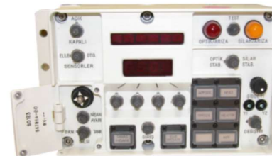
Fire Control Computer with BMS Interface
